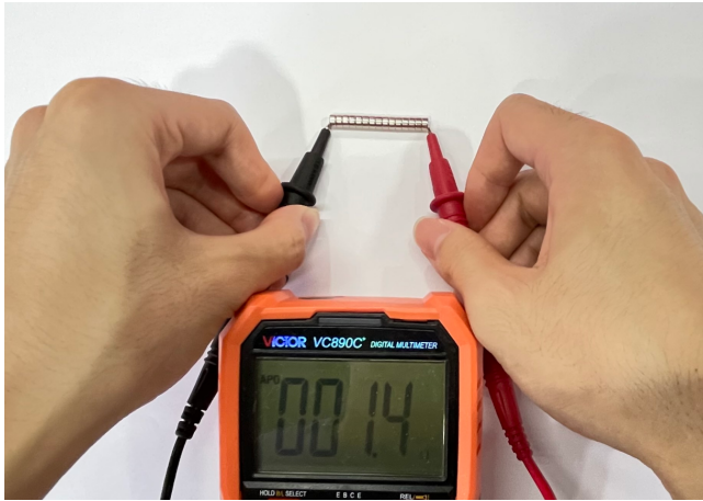
Figure 3: A resistance test on neodymium magnets: we conducted several tests on 15 neodymium magnets with a diameter of 5mm and a thickness of 3mm, and the results showed that the resistance of the 15 neodymium magnets was 1.4\Omega
